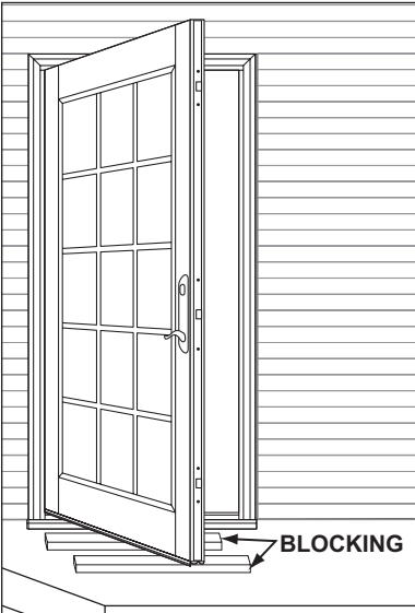
FIGURE 2 Outswing Hinge Viewed From Interior
